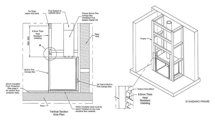
Figure 2: Woodburner diagrams from the manufacturer's specification (not to scale)
