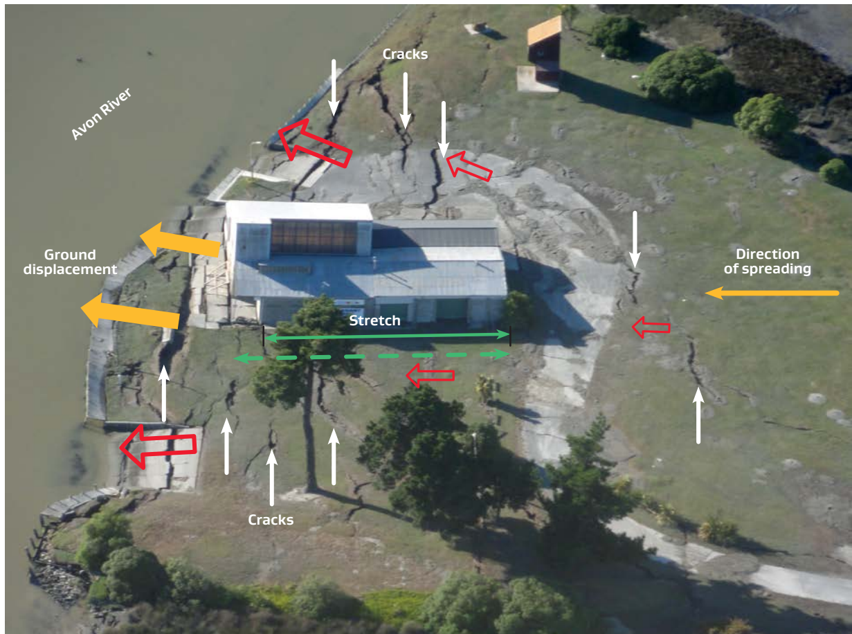
Figure 5.4: Characteristic features and effects of lateral spreading illustrated on a Christchurch case history (modified from Cubrinovski (2019), Ralph B. Peck Lecture)
