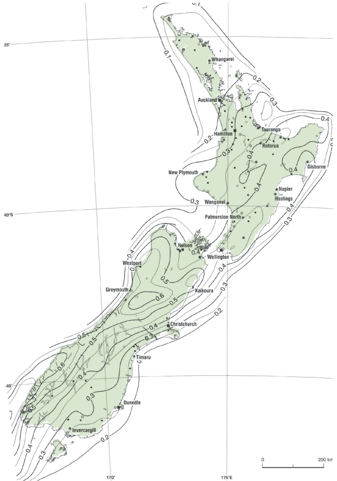
Figure A.2: Unweighted peak ground acceleration coefficients, C_{0,1000} corresponding to a 1000 year return period at a subsoil Class D or E deep or soft soil site
