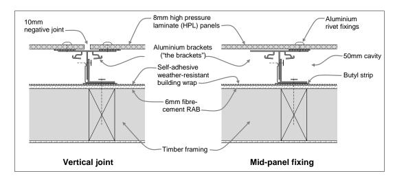
Figure 1: Typical construction of the original façade system (not to scale)
